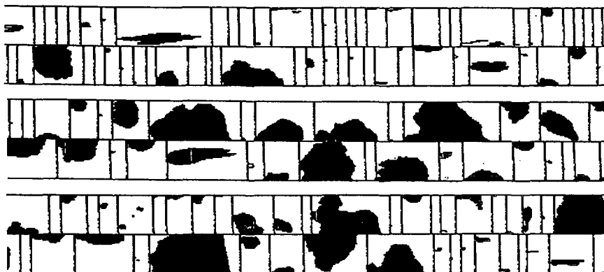
FIG. 10. Graupel images from an optical array spectrometer probe recorded from 2116:02 to 2116:16 as N10UW penetrated the echo on the western edge of the BWER. The distance between horizontal lines is 800 \mu\text{m} and the vertical lines between images are coded time bars.
